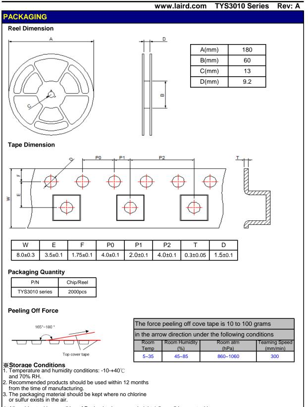
4. Allowable stacking condition of Packaging box: max height 1.5m or 5 boxes stacking
