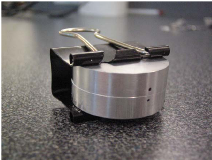
Picture #2 Aluminum disks clamped with PCM between them
