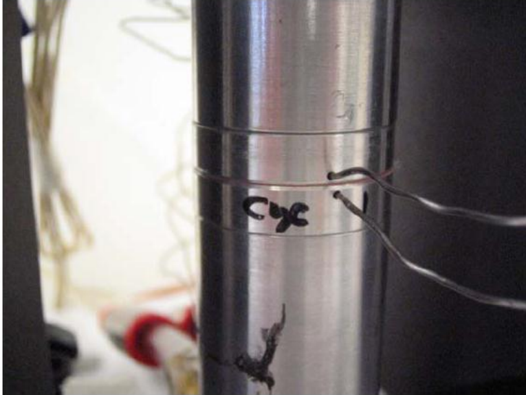
Picture #3 Close-up of the aluminum disks in the thermal tester
