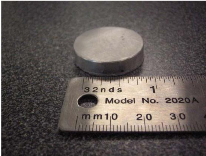
Picture #1 Aluminum disk used for reliability testing
