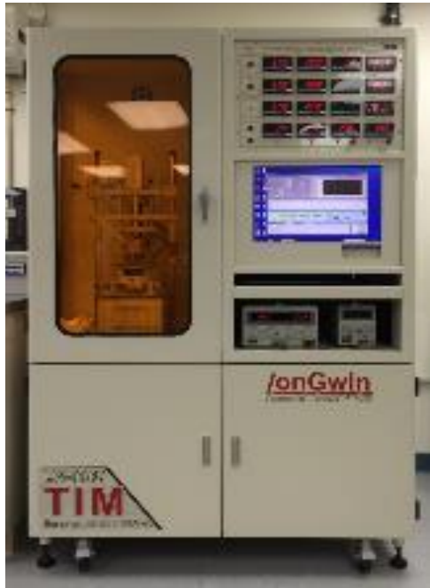
Figure 3: LonGwin ASTM D5470 Thermal Resistance Tester
