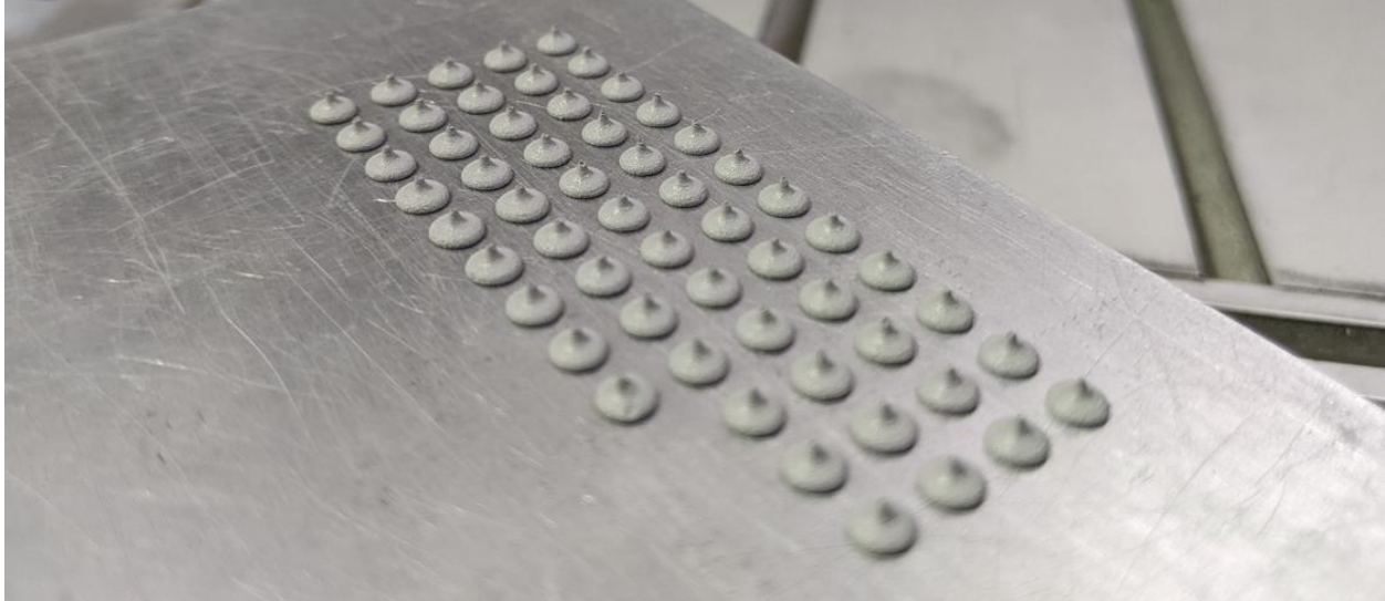
Volumetric dispensing can achieve fast, repeatable, small dots, such as these 3.5-mm dots with volume 0.0078 cm 3 , dispensed using an 18-gauge needle (ID = 0.84 mm).
