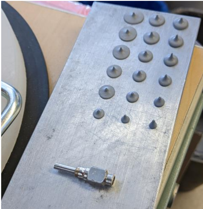
Volumetric dispensing can achieve fast, repeatable, small dots, such as these 3.5-mm dots with volume 0.0078 cm 3 , dispensed using an 18-gauge needle (ID = 0.84 mm).
