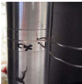
Close-Up of The Aluminum Disks in the Thermal Tester
