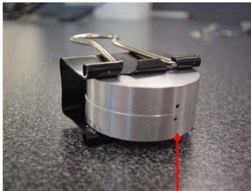
Thermocouple location Aluminum Disks Clamped with Sample
