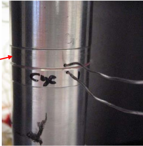
Figure 7: Close-Up of The Aluminum Disks in the Thermal Tester
