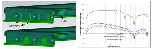
There are more cases proving that the long-side dimension of the aperture plays a decisive role in the shielding effectiveness, regardless of the short-side dimension. Therefore, in practical application, engineers should avoid some long slit aperture designs, even if the gap width is small.
