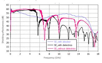
graph. With absorber material attached inside, the BLS becomes a loss cavity. The resonance points are all removed. This is the typical application for a BLS and absorber combined
